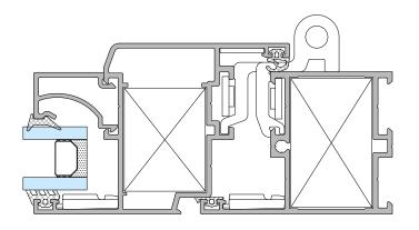
This lightweight budget-friendly system; is a hinged window and door system without heat barrier that is used in places where strong systems are not needed and looks elegant with its thin appearance.
