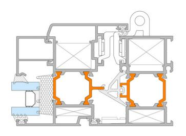
As aluminum conducts heat and cold, Skyprof offers the thermally improved S65 aluminum window and door series. A heat barrier is used in this system to thermally separate the inner and outer surfaces.
