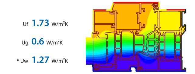
\* Calculated according to EN 10077-2:2017 on a 1230x1480 mm one sash window with Ug=0.6 W/m<sup>2</sup>K glass.
